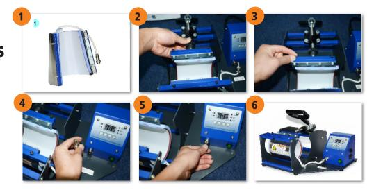
Before changing heater bands make sure that the power is switched off and the machine is cool. Changing heater bands;
